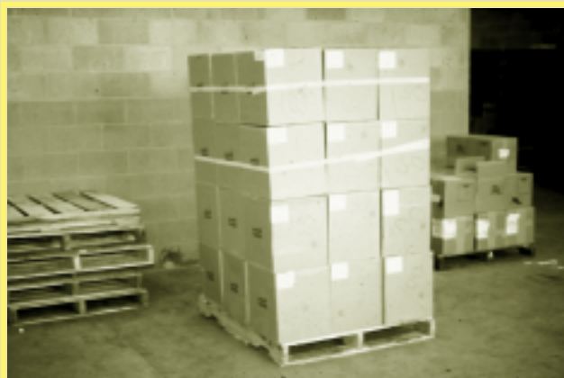
Figure 1. — A typical unit load for the storage and distribution of consumer and industrial products.
